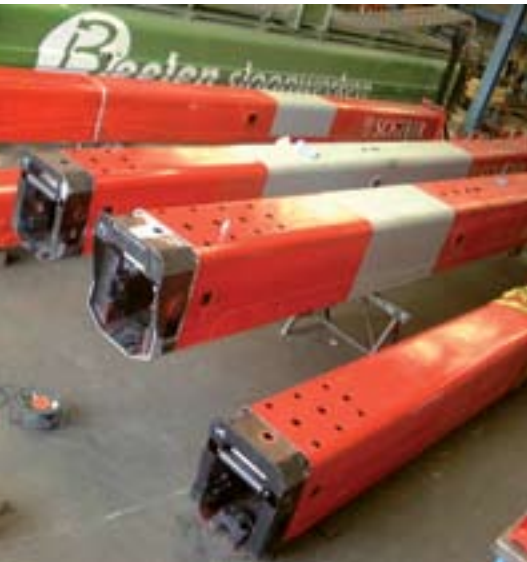
Telescopic boom sections in for repair at Rusch Kraantechnik in the Netherlands
