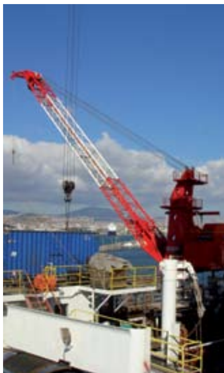
This Liebherr BOS 30/3000 was one of three offshore cranes refurbished by Liebherr-Werk Nenzing for a customer in Istanbul, Turkey
