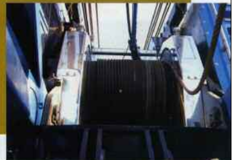
Stainless steel is used to replace non-structural steel parts on Lampson's Manitowoc cranes as part of the refurbishment programme
