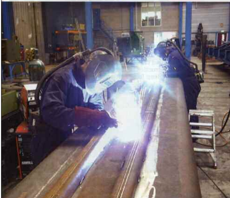
Rusch Crane Repair welders working on a telescopic boom repair
