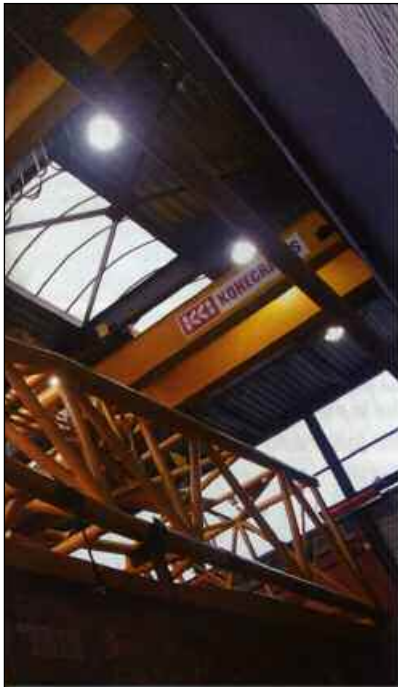
A lattice boom section awaiting repair in Avezaat's Dutch facility
